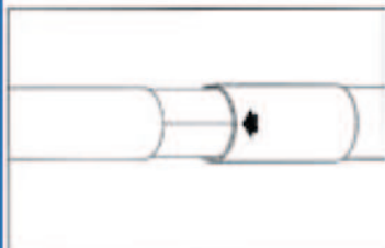
3) Place the shrinking socket on the jointing area covering evenly the ends of the pipes.
